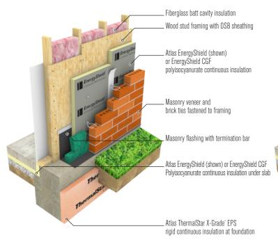
IMAGE 2: WOOD FRAME WITH LATERAL BRACING, ENERGYSHIELD WITH BRICK VENEER OR EXTERIOR SIDING
