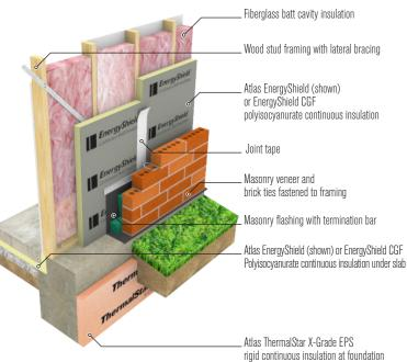
Note #3: For multiple layer EnergyShield/EnergyShield CGF installations, offset vertical joints between first and second layers of EnergyShield/EnergyShield CGF by at least one stud cavity and horizontal joints by at least 152 mm (6 inch).
